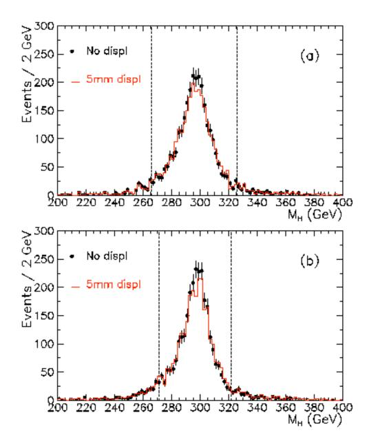
Figure 7: The effect of 5 mm longitudinal displacement of one EC on the reconstructed  $300 \text{ GeV/c}^2 \text{ Higgs}$  mass (a), and on the fitted one using a Breit-Wigner Z mass constraint (b). The lines indicate the mass windows used in each case.
