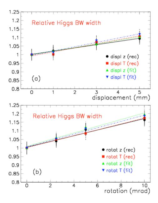
Figure 8: The relative increase of the width of the reconstructed or fitted 200 GeV/c<sup>2</sup> Higgs as a function of the size and type of translation (a) and rotation (b). The lines correspond to linear fits showing the trend of the increase.
