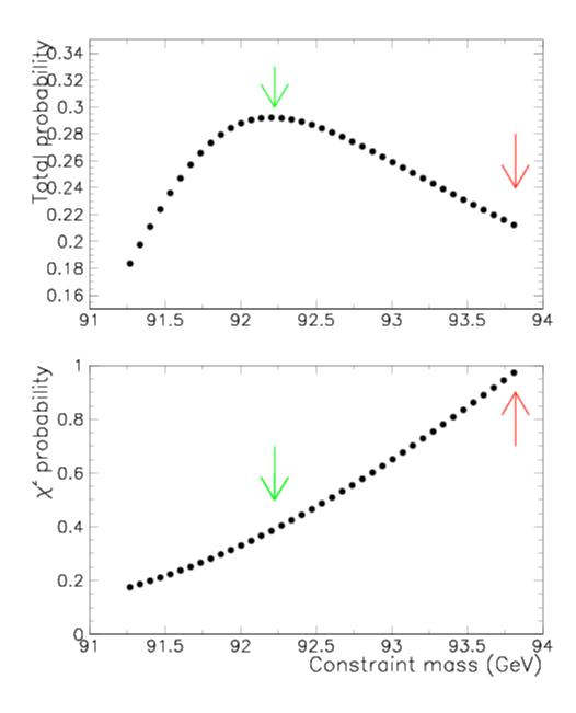
Figure 2 a) and b) show the probability and the  $\chi 2$  respectively as a function of the dimuon mass for a typical event. With green arrow we indicate the initial unfit mass value and with red arrow, the fit value.
