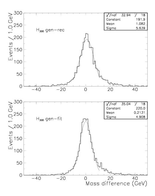
**Figure 5**: shows the reconstructed minus the generated Higgs mass before and after the constrained fit described in the text. The generated Higgs had a  $300~\text{GeV/c}^2$  mass.
