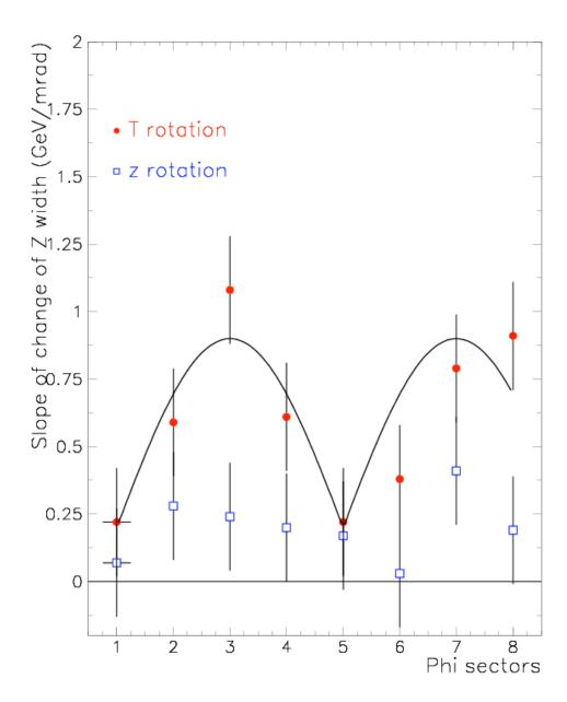
**Figure 14:** The modulation of the slope of the increase of the width of the reconstructed **Z** mass as a function of phi, for rotations around the x axis (red circles) and the z axis (blue rectangles).
