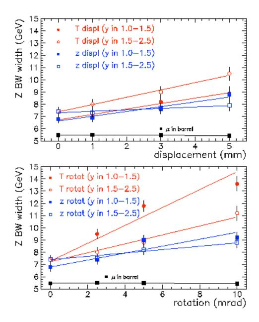
**Figure 13:** The relative increase of the width of the reconstructed **Z mass** as a function of the size and type of translation (a) and rotation (b). The lines correspond to linear fits showing the trend of the increase. At least one muon was required to be reconstructed in the misaligned area. The case where both muons are in the barrel is also shown for comparison.
