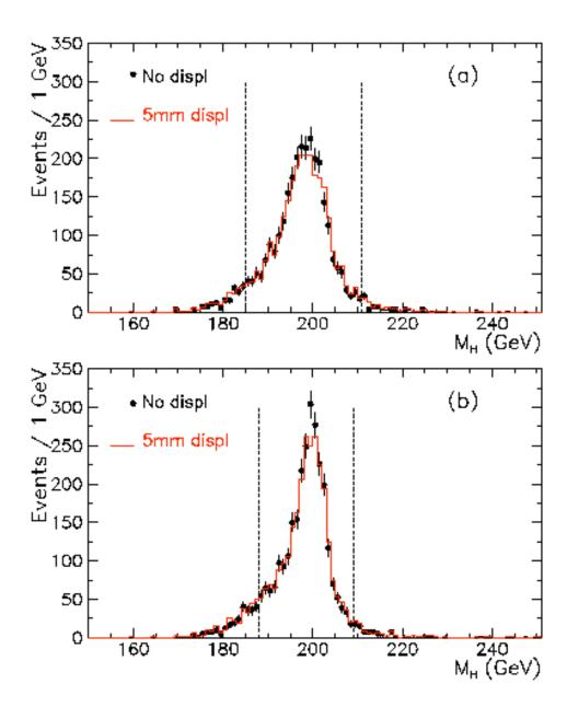
Figure 6: The effect of 5 mm longitudinal displacement of one EC on the reconstructed 200 GeV/c<sup>2</sup> Higgs mass (a), and on the fitted one using a Breit-Wigner Z mass constraint (b). The lines indicate the mass windows used in each case.
