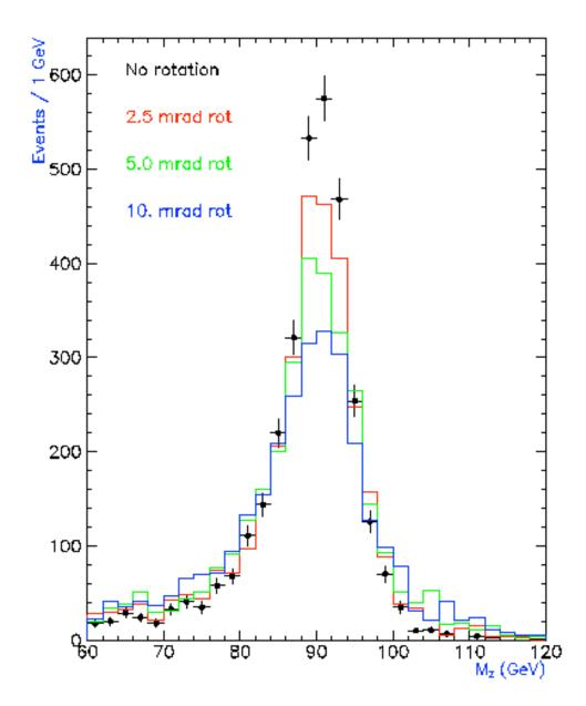
**Figure 12:** The effect of 2.5, 5 and 10 mrad rotation- of all sectors belonging to one EC, around the ATLAS x- axis- on the reconstructed **Z** mass.
