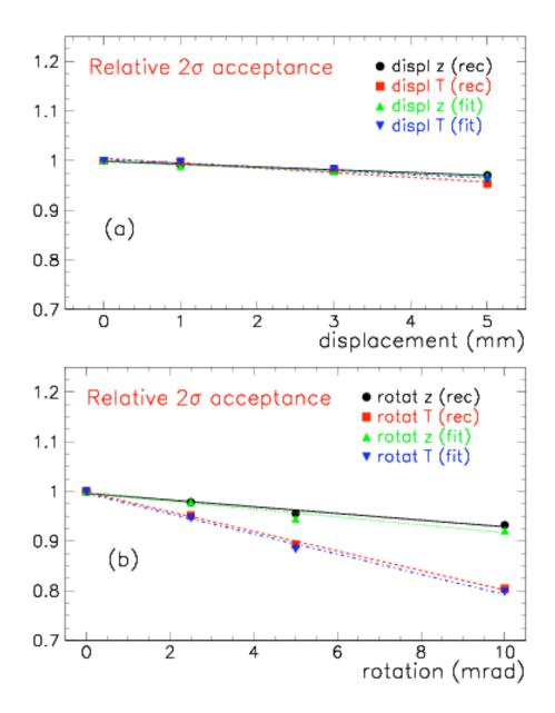
Figure 9: The relative decrease of the number of accepted, reconstructed or fitted 200  $GeV/c^2$  Higgs as a function of the size and type of translation (a) and rotation (b). The lines correspond to linear fits showing the trend of the decrease.
